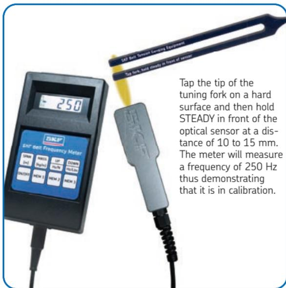
Tap the tip of the tuning fork on a hard surface and then hold **STEADY** in front of the optical sensor at a distance of 10 to 15 mm. The meter will measure a frequency of 250 Hz thus demonstrating that it is in calibration.
